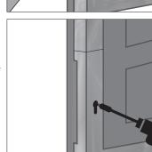
• Drill Two holes using a 17mm and 5mm drill bit from the outside of the door until they almost penetrate the inside surface of door. Then finish the hole by drilling from the inside of the door. Carefully chisel out the cylinder shape as determined by the template.
